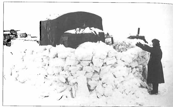
A German truck driver tries to shelter his truck from the extreme cold of the icy Russian winter. The very low temperatures meant that ordinary engine oils would simply freeze solid without the use of special additives or would force the crew either to keep the engine running, something that was wasteful on fuel, or light a fire under the engine to thaw it out. (IWM, HU5180)
