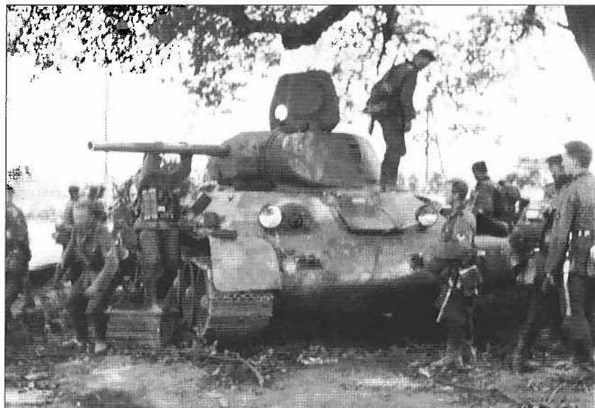
German infantry inspecting what appears to be an abandoned T-34/76. The first few times these tanks appeared they caused panic as the standard 3.7cm anti-tank gun could not penetrate the armour. The 5cm anti-tank guns fared better but often the Germans would improvise using the 8.8cm gun in an antitank role. (Nik Cornish Library)
