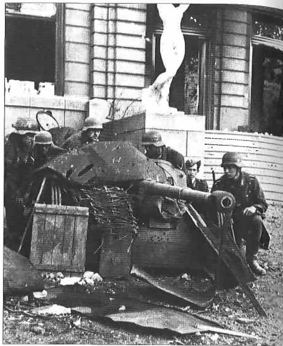
Luftwaffe ground troops with a partially camouflaged PAK 38 anti-tank gun, possibly defending one of the airfields around Stalingrad. The successor to the PAK 36, it used a larger calibre (5cm) round that was more effective against the heavier Soviet tanks, such as the KV-1 and T-34, penetrating up to 76mm of armour at 500m. (IWM, HU5168)
